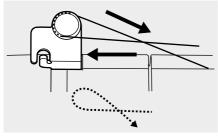
3. Wind the thread clockwise around the bobbin winder tension discs.
