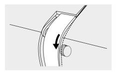
Thread the tension module by passing the thread between the silver discs.
