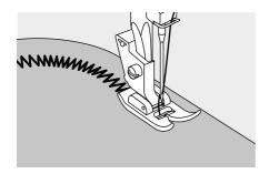
When sewing along a curve while using a zigzag stitch, select a shorter stitch length in order to obtain a finer stitch.
