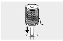
Place the thread and spool holder onto the spool pin.
