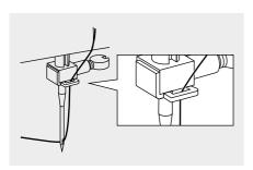
8. Now pass the thread behind the thin wire needle clamp guide. Pull the end of the thread through the needle from front to rear and pull out about 10 cm of thread. Use the needle threader to thread the needle.
