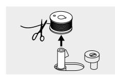
9. Cut the thread and then remove the bobbin.
