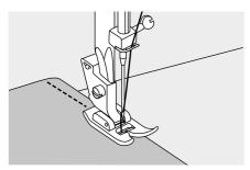
Lower the presser foot lifter and then press the foot control to start sewing.
