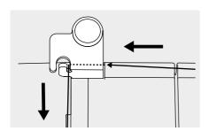
4. Guide the thread around the thread guide as illustrated.
