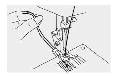
Lay both threads to the back under the presser foot.
