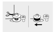
After the bobbin has wound a few turns stop the machine and cut the thread near the hole of the bobbin.
