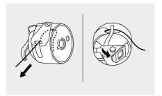
Pull the thread through the slit and under the finger.
