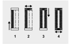
Follow the 4-step sequence changing from one step to another with the pattern selector dial. When moving step by step through the buttonhole process, be sure that the needle is raised before turning the pattern selector dial to the next step. Take care not to sew too many stitches in steps 2 and 4. Use the seam ripper and cut the buttonhole open from both ends towards the middle.
