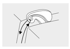
7. At the top of this movement pass the thread from right to left through the slotted eye of the take-up lever and then downwards again.
