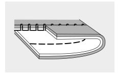
Thread tension is too tight for straight stitch sewing. Turn the dial to the lower number.
