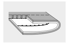
Thread tension is too loose for straight stitch sewing. Turn the dial to the higher number.
