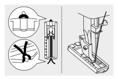
Attach the buttonhole foot and hook the gimp thread onto the back of the presser foot.
