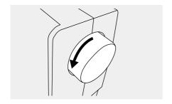
Raise the needle to its highest position by turning the handwheel towards you (counterclockwise) . Raise the presser foot to release the tension discs.
