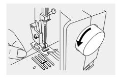
Hold the upper thread with the left hand. Turn the handwheel towards you (counterclockwise) lowering it, then raise the needle.
