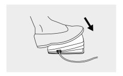
7. Press on the foot control to start winding the bobbin.
