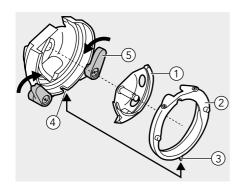
Replace the hook. Attach the hook race cover making sure the bottom pin fits into the notch. Snap back the two hook retaining arms. Insert the bobbin case and bobbin and replace the stitch plate.
